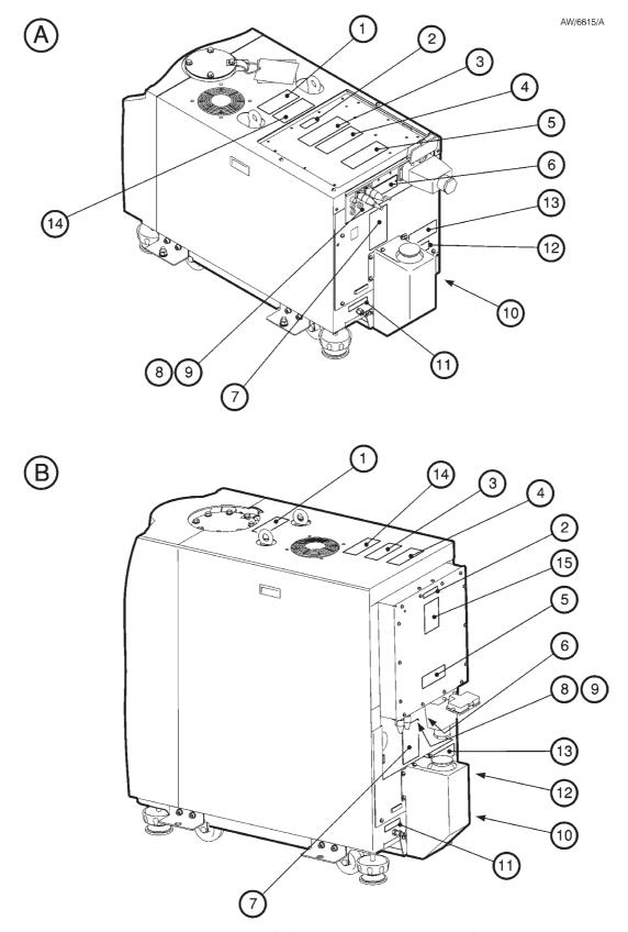
Figure 1-11 - Label positions on iH system enclosures
