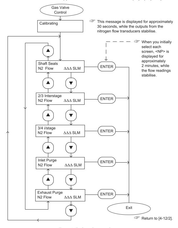
Figure 4-15 - Gas valve control menu
