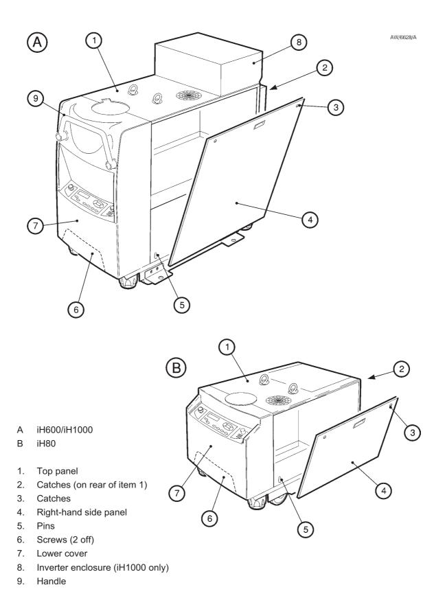
Figure 3-3 - Remove/refit the enclosure panels
