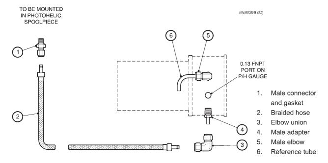
Figure 3-16 - Photohelic gauge piping connections
