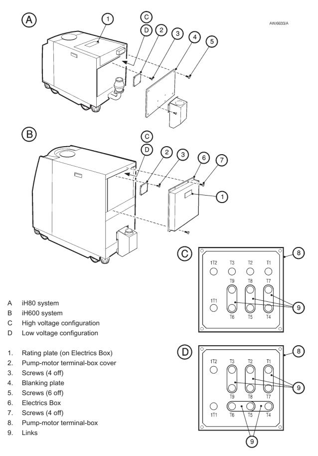
Figure 3-9 - Reconfigure the pump-motor terminal-boxes (iH80/iH600 only)
