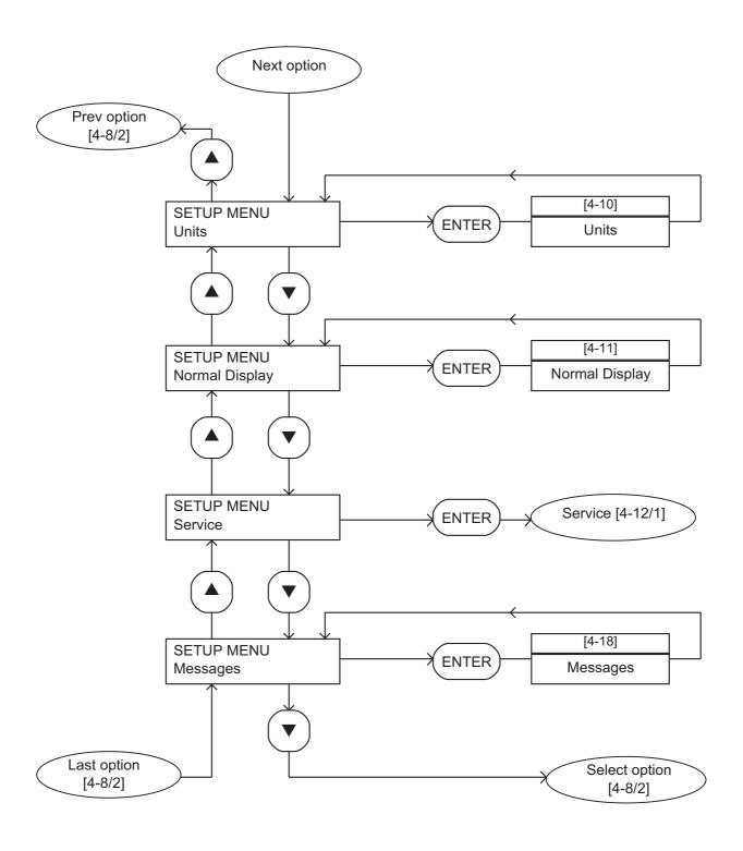
Figure 4-8 - Setup menu: sheet 3 of 3
