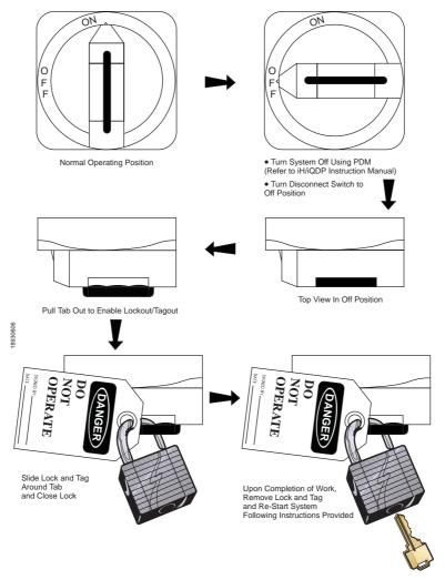
Figure 6-6 - System lockout/tagout procedures
