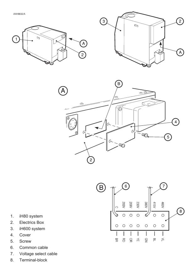
Figure 3-8 - Reconfigure the iH system for your electrical supply (iH80/iH600 only)
