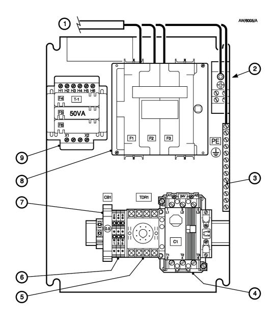
Figure 3-13 - Disconnect box sub-panel general arrangement
