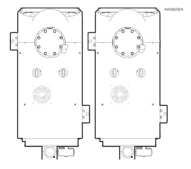
Figure 3-5 - System arrangement to reduce effective footprint (if required)
