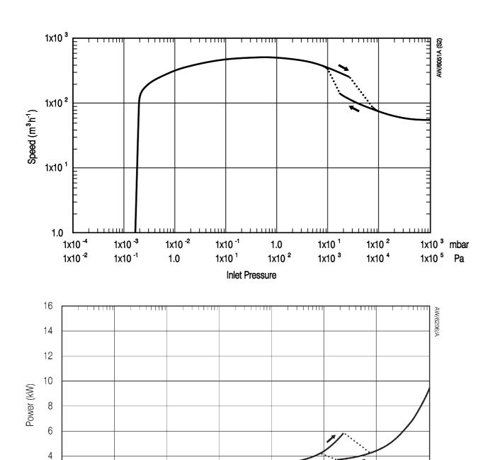
Note: Discontinuity in curves are as a result of the HCMB pressure relief valve opening and closing
