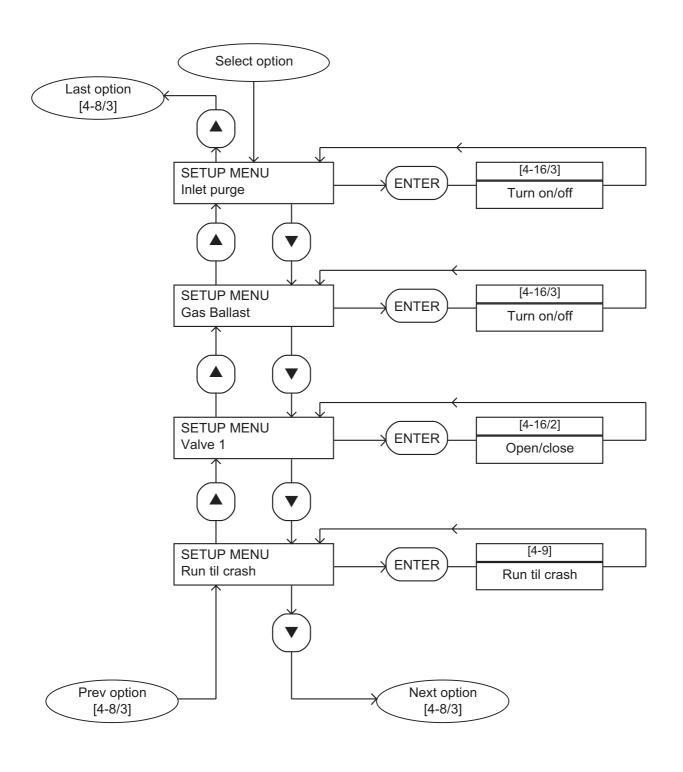
Figure 4-8 - Setup menu: sheet 2 of 3
