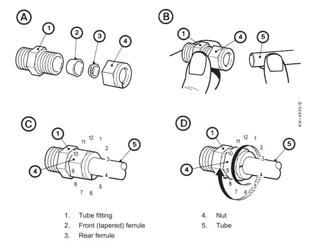
Figure 6-1 - Fit a tube fitting
