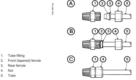
Figure 6-2 - Retighten a tube fitting
