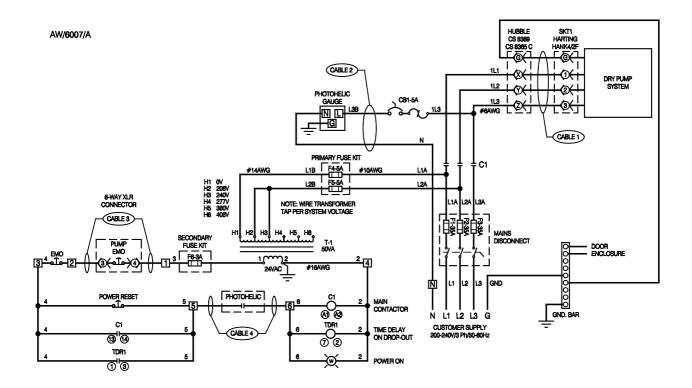
Figure 3-12 - Disconnect box electrical schematic
