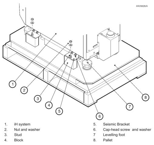
Figure 3-1 - Remove the iH system from the pallet
