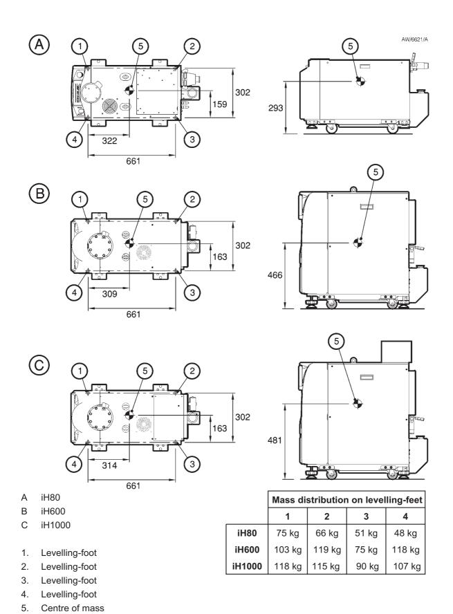
Figure 2-5 - Centres of mass dimensions (mm) and mass distribution
